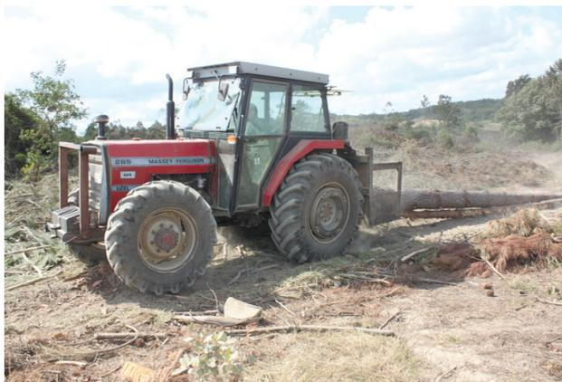
**Figure 2.** Skidding logs by farm tractor.
